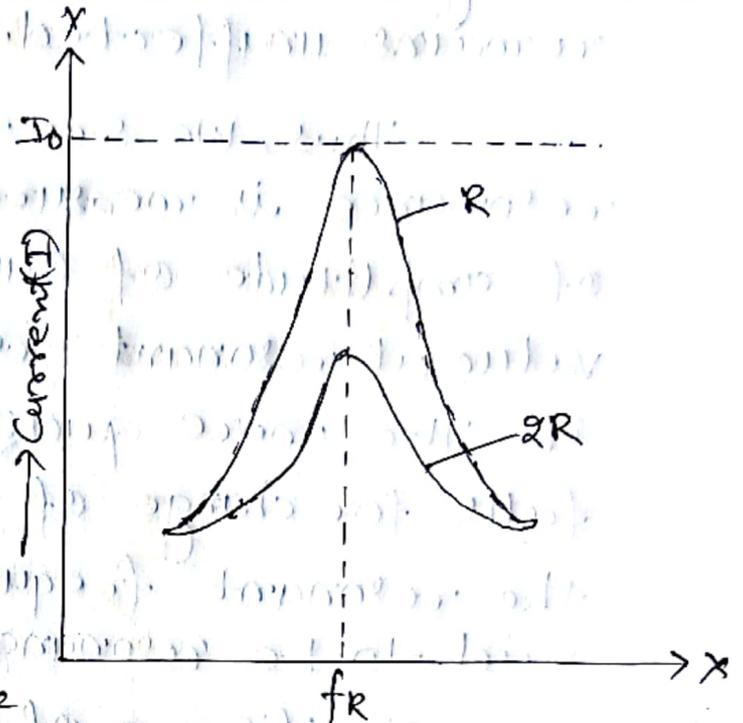
figure. At first, the current is very small increases to a maximum when the frequency increases to its resonance value  $f_r$  and then falls again. Before resonance the current lags behind the applied e.m.f. at resonance it lags behind the e.m.f.
